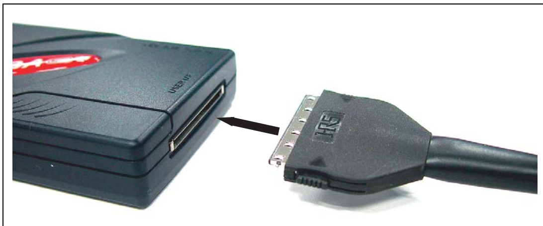
Figure 2.2 Connecting the E10A-USB Emulator to the User System Interface Cable
